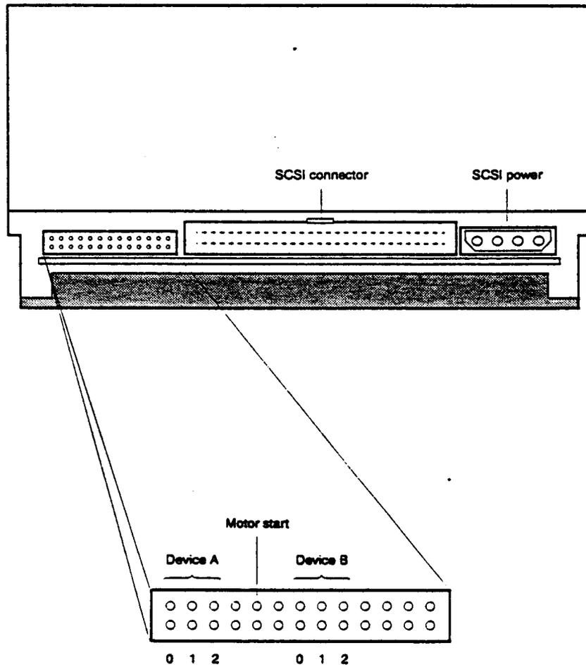
**Note:** This disk drive consists of two 3.5" hard disk assemblies (HDAs) and a PCA controller, which are configured in a 5.25" enclosure. Each HDA (device A and device B) must be assigned a unique SCSI address (drive ID).
