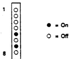
7. After the system has boot the IRIX operating system, the CPU LEDs display the following pattern during normal operation:
