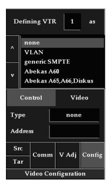
[ ] 8. Click on the green **Config** button. The message Initializing VTRs will appear followed by Done Initializing VTRs. Note that if the recorder is off the network, IRIX will try connecting for 90 seconds before reporting a failure.
